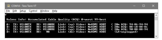
The picture is using a 4-channel card as example. If you have a 6-channel card, channels A-F will be displayed.
