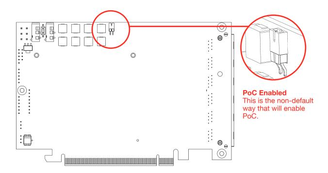
+ Note: Power over Cable will enable 24V 0.5A on each of the RJ45 connector channels.
